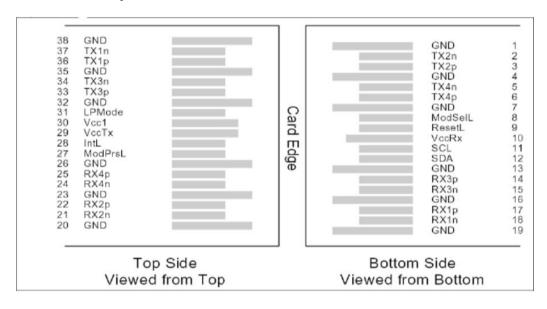
Figure 1 - QSFP28-Compliant 38-Pin Connector
