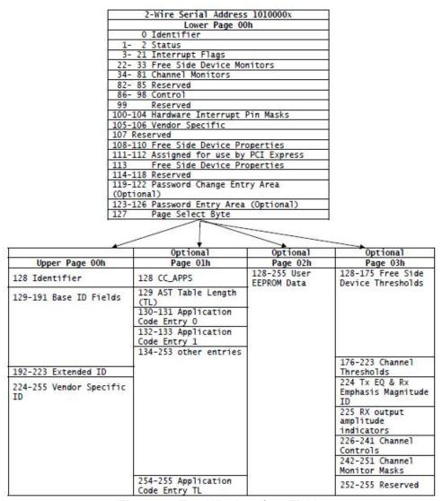
Figure 2 - Two-Wire Interface Fields
