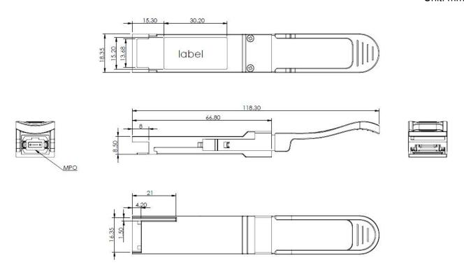
To minimize MPO connection induced reflections, an MPO receptacle with 8-degree angled end-face is utilized for this product. A female MPO connector with 8-degree end-face should be used with this product as illustrated in below.
